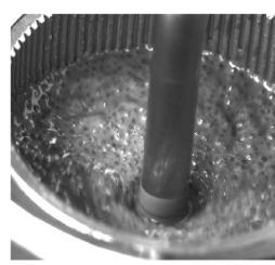
Mortar SRM in rheometer
