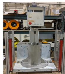
A Concrete Rheometer
