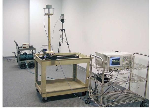
Fig. 2. The measurement system using a vector network analyzer and a virtual circular antenna array. (a) Block diagram; (b) photograph.
