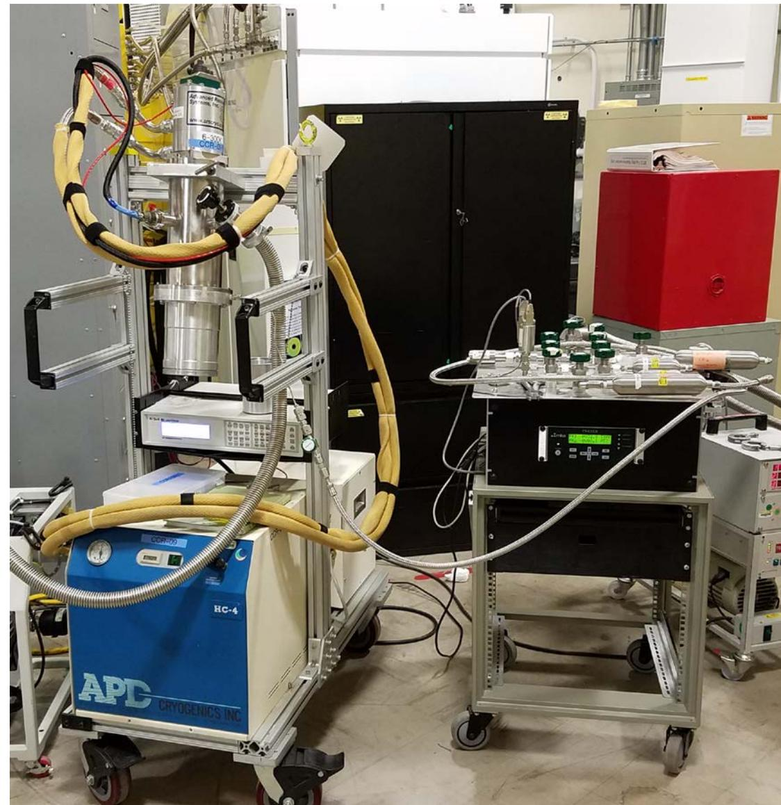
CCR attached to CO<sub>2</sub> line for gas dosing
