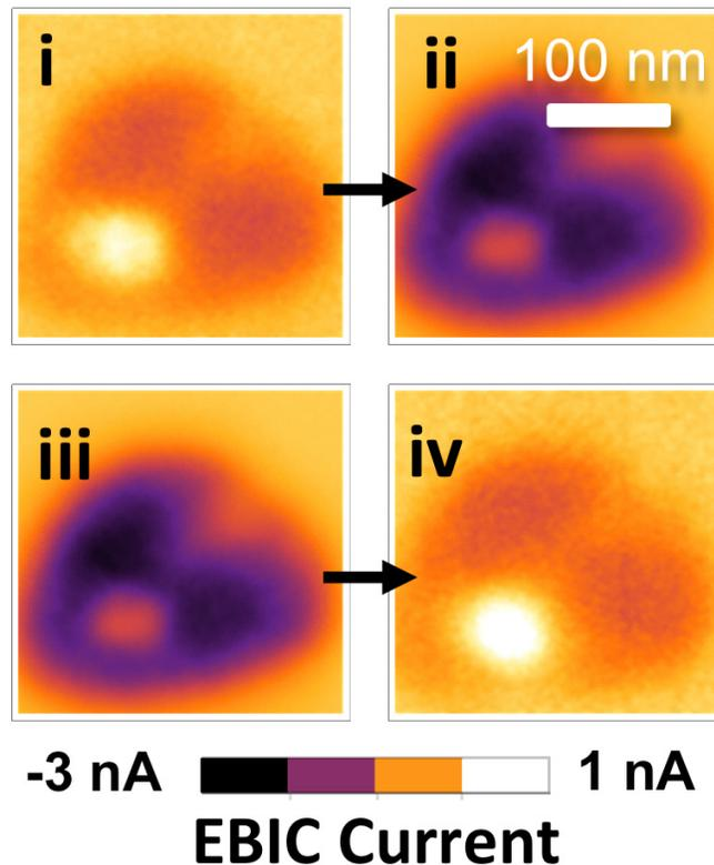
Electron Beam Induced Current Micrographs of a memristor, showing switching from a state of low resistance (i) to high resistance (ii), and from high resistance (iii) back to low resistance (iv) again. The bright resistive switching core is surrounded by a darker region that indicates a path where current may leak out, reducing performance of the memristor. Credit: CNST
