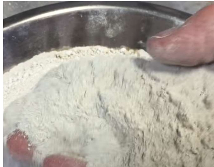
Ground gypsum from clean job site construction dry wall gypsum waste
