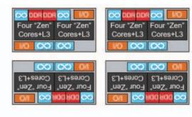
4 x 8-core Chiplet, 213mm<sup>2</sup> per chiplet 852mm<sup>2</sup> total area (+9.7%) 0.59x Cost
