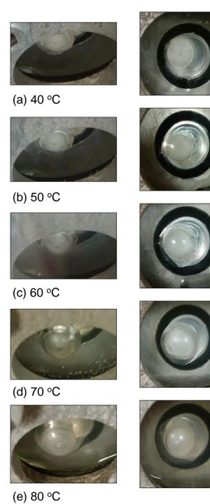
Figure 5. Results of a thermal blister test on an EVA-glass sample. The water was heated in intervals of 10 °C, starting at 40 °C. Between each increase, the sample was allowed to thermally equilibrate for 45 minutes. The photographs show the blister "ballooning"—i.e. deforming mechanically, significantly—while the blister grew slightly. This seems to indicate that the EVA-glass adhesion was strong, compared to the stiffness of the EVA.
