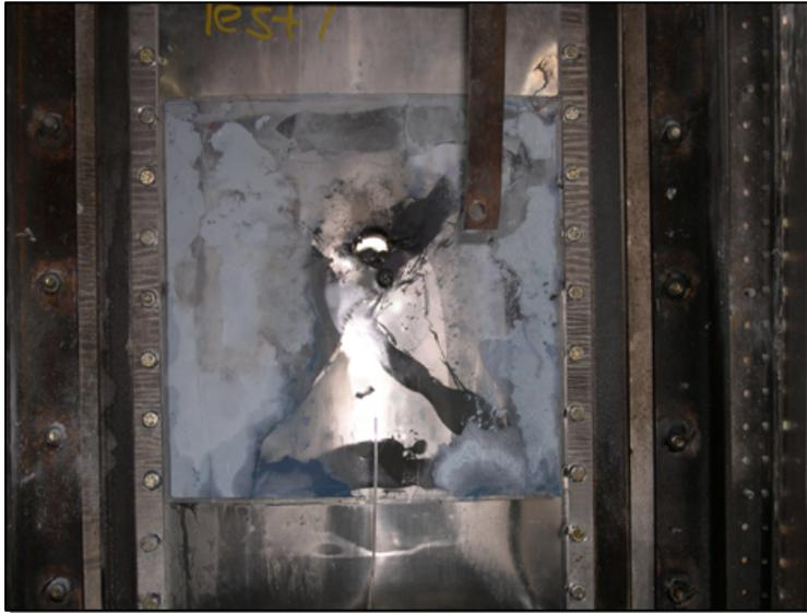
**Figure 9–30. Post-Test Damage Image of EPP-07 Enhanced Powder Panel.**
