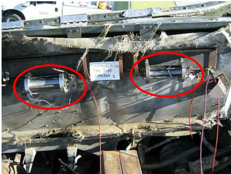
**Figure 9–45. SPGGs Installed in Mid-wing Test Article for Live-fire Demonstration.**<sup>47</sup>
