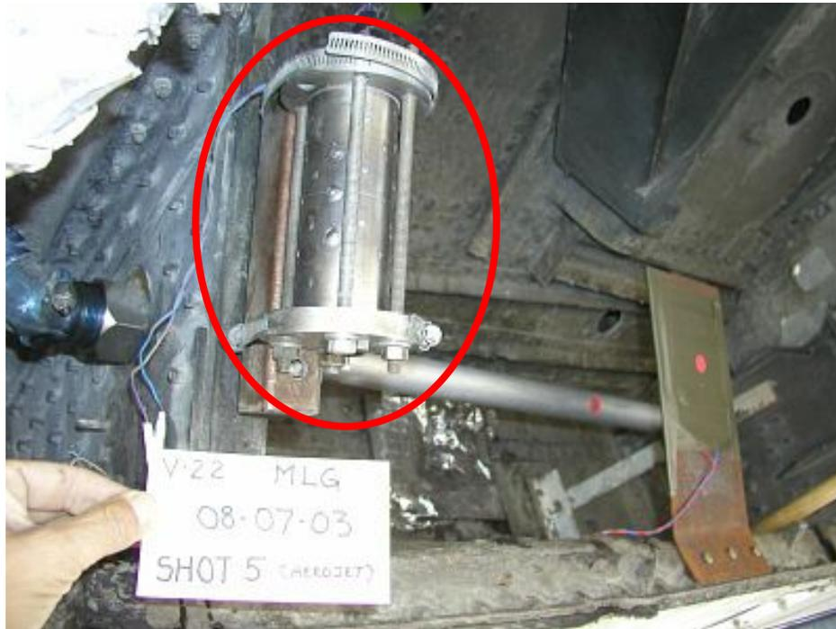
**Figure 9–44. SPGG Installed in Sponson Test Article for Live-fire Demonstration.**<sup>46</sup>
