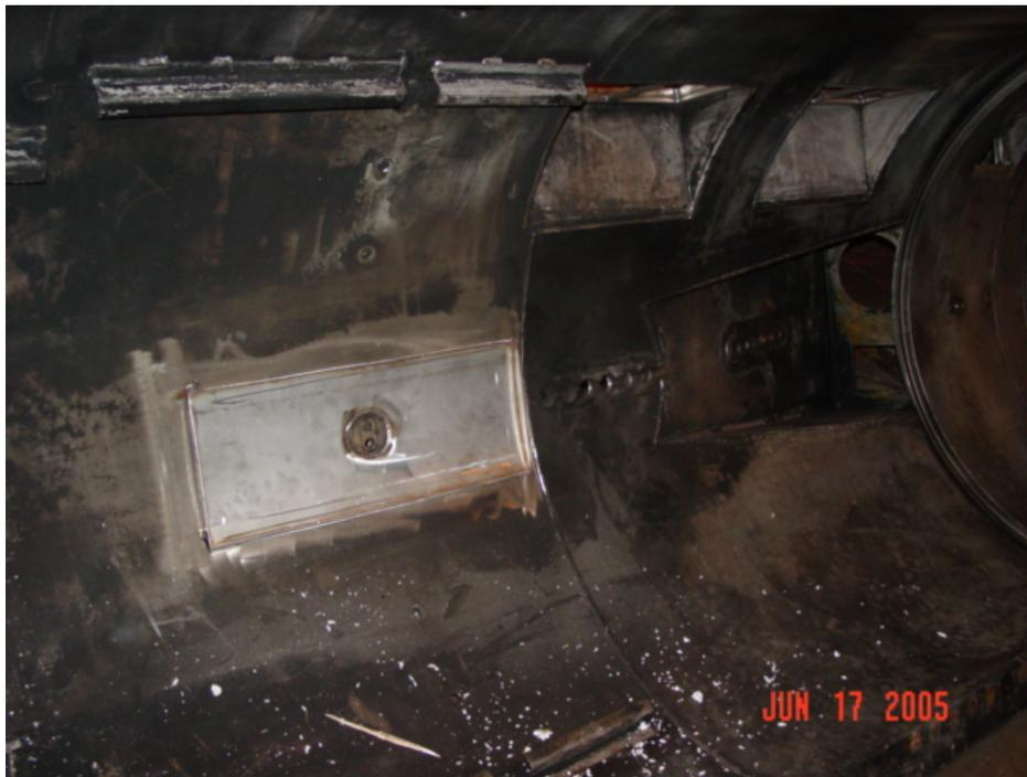
**Figure 11–7. Pool Fire Pan in Nacelle.**
