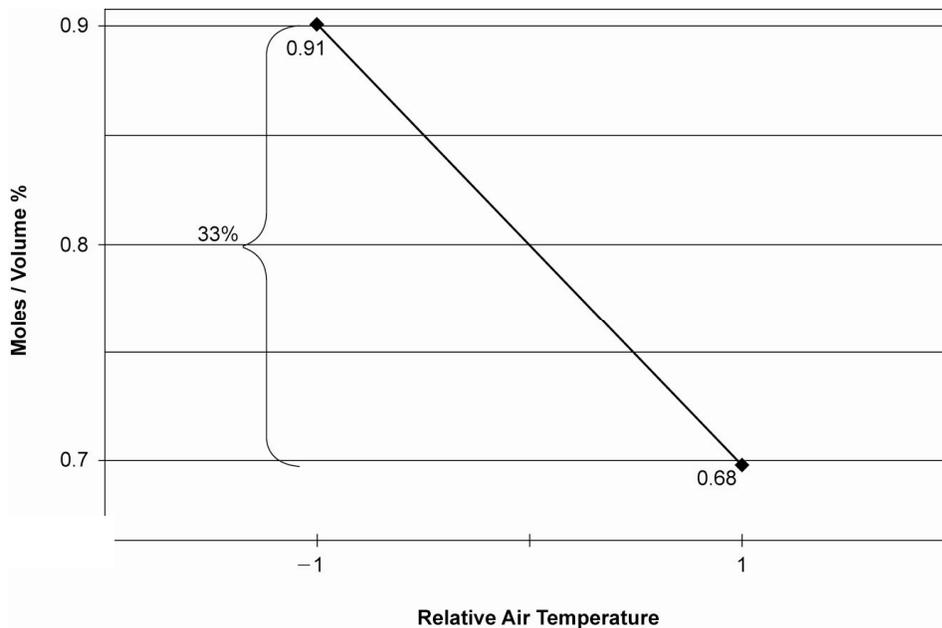
**Figure 11-15.** Variation of Moles of Injected Chemical per Fire Zone Volume Percent with Relative Air Temperature. (“-1” is 10 °C below the agent boiling point; “1” is 60 °C above the agent boiling point.)
