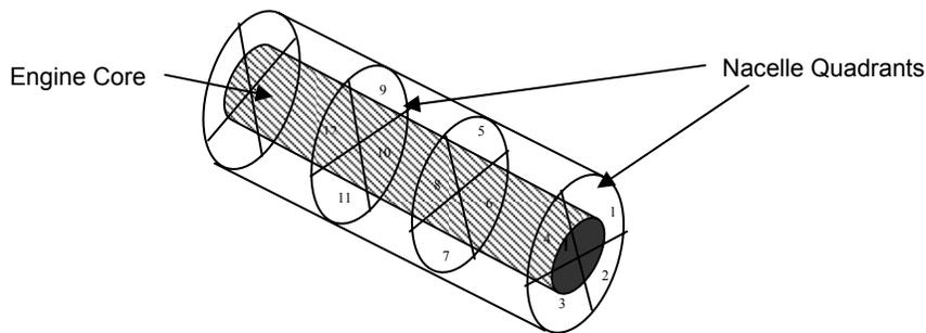
**Figure 11–13. Phase II Nacelle Concentration Measurement Quadrants.**
