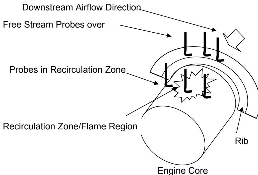
**Figure 11–11. Halonyzer Probe Mounting in Flame Region.**
