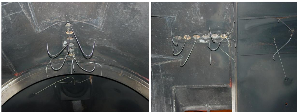
**Figure 11–12. Halonyzer Probes in Nacelle Fixture.**
