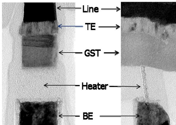
Phase Change Memory Stacks requiring good characterization of heater resistivity and phase change material characterization
