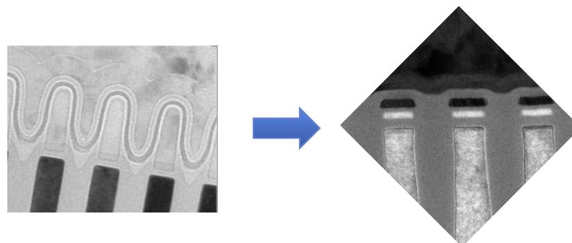
Even if physical limitations are resolved, reliability of such devices is a challenge 1xnm NAND technology node is challenged by >50% interference, E-fields at breakdown limits, & disturb issues
