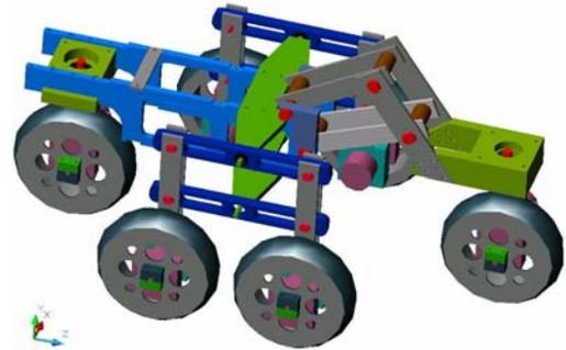
Fig.3. CAD model of the modified Shrimp Rover
