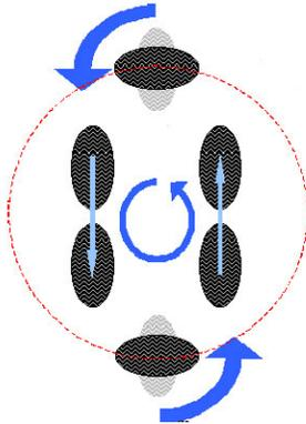
Fig.9. Turning of robot
