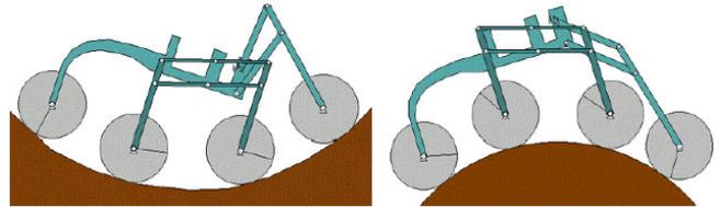
Fig.4. Robot flexibility in Convex/Concave environment.
