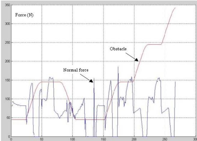
Fig. 16. Back wheel force diagram during obstacle crossing
