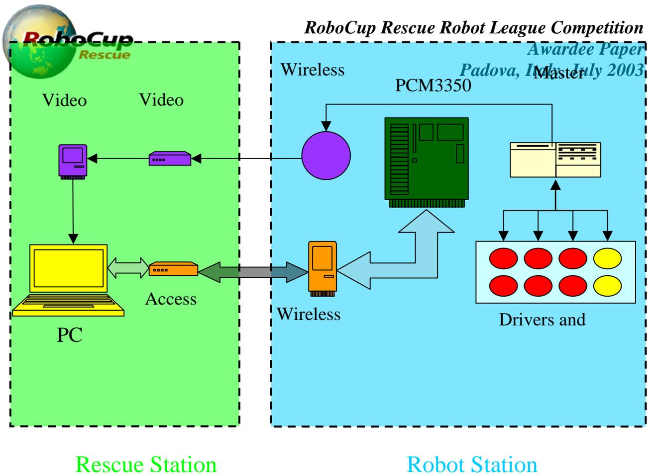
Fig. 19. The communications and control units
