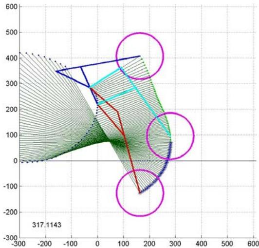
Fig.11. Front fork mechanism used in Shrimp Rover (all dimensions are in mm)
