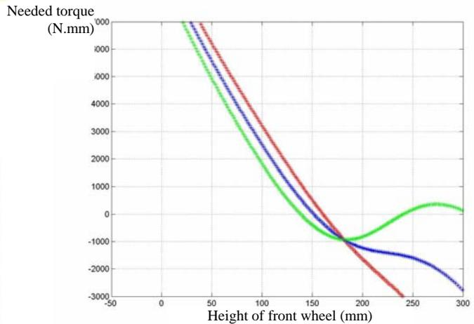
Fig.15. Torque needed for climbing for three different springs
