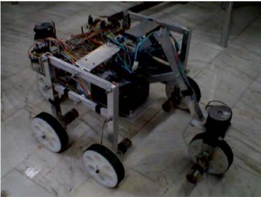
Fig.1. Alpha prototype of the Shrimp Rover
