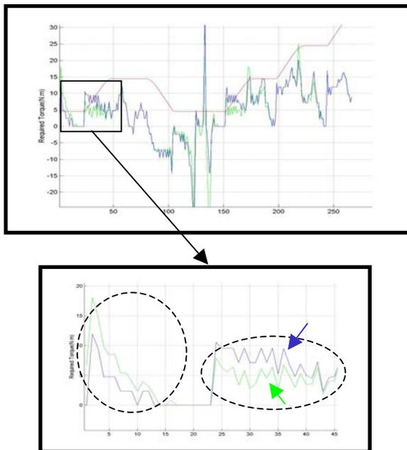
Fig. 17 Needed torque to provide energy in two cases: with and without the spring
