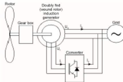
Doubly-Fed Machine can sink or sources VARs, with high bandwidth control
