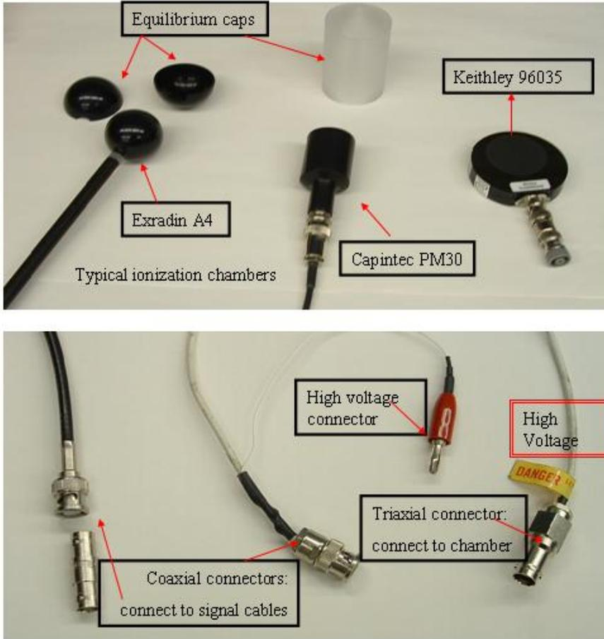
Figure 4. Typical chambers and connectors.
