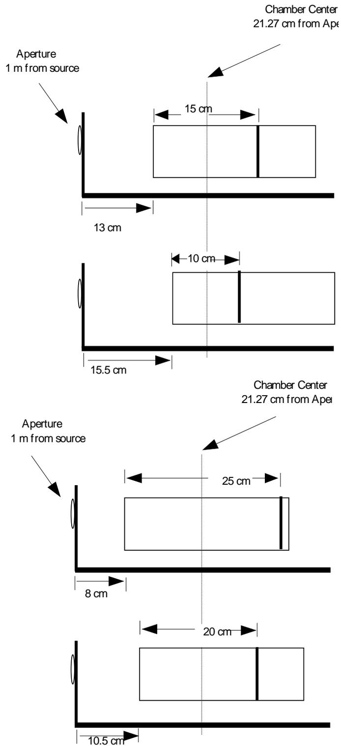
Figure 2. Typical Attix chamber configuration for air-kerma measurements.
