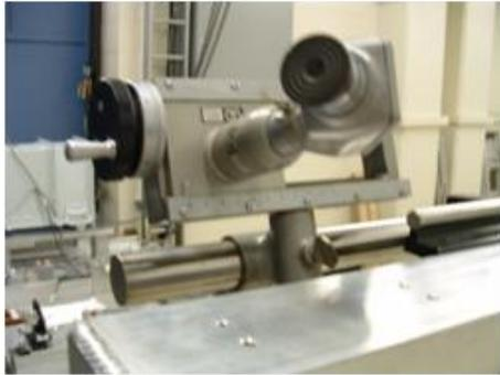
Alignment telescope 300 kV range
