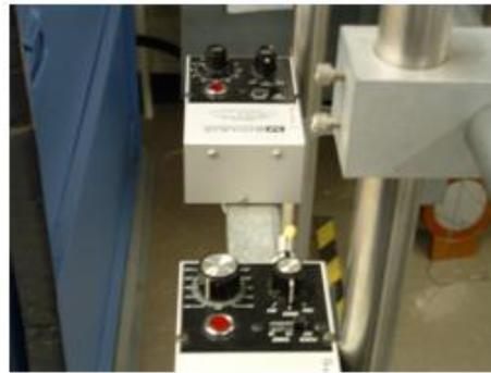
Chamber alignment controls 100 kV range
