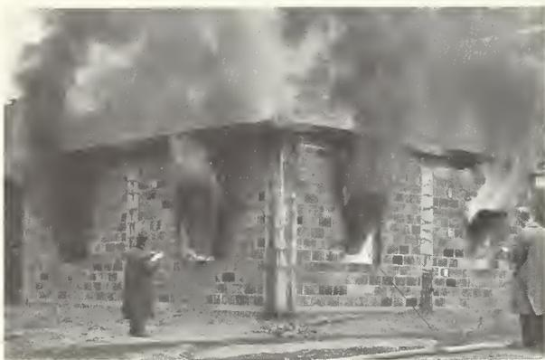
*Measuring the duration and intensity of a fire during a burnout test simulating a severe fire in a storage warehouse, with known amounts of combustible loading on the interior. Tests of this type determine the temperatures to which it is proper to subject building materials and constructions in fire test furnaces, and serve as a guide in applying the results of such furnace tests to building design.*
