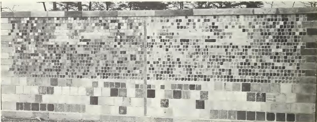
*A test wall, comprised of 2352 samples of building stone supplied by 47 states in the U.S.A. and 47 foreign countries, was constructed on the Bureau grounds in 1948 to study the nature and rate of deterioration of the different stones. Structural features such as length changes, warpage, back waterproofing, and grade waterproofing were also observed in relation to weathering and discoloration.*
