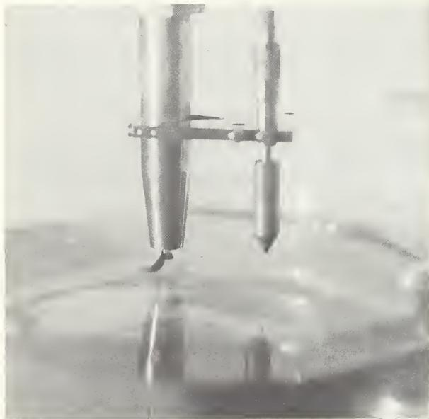
*The parameters controlling backflow of water from a lavatory across an air gap into a faucet, illustrated in this figure, were studied to obtain critical values. Backflow can occur from a lavatory into an open faucet when unusual conditions produce a vacuum in the water system, if the faucet overhangs the rim of the lavatory improperly.*
