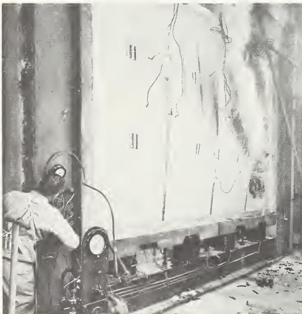
*Fire endurance test of a prefabricated lightweight wall panel designed for use in arctic regions. This photograph shows the unexposed surface 55 minutes after the fire exposure started and shortly after flames broke through a joint. Initial failure, at 45 minutes, was due to excessive temperature rise as measured by thermocouples mounted under asbestos pads. The panel continued to support the structural load, applied by jacks at the bottom, throughout the duration of the test.*
