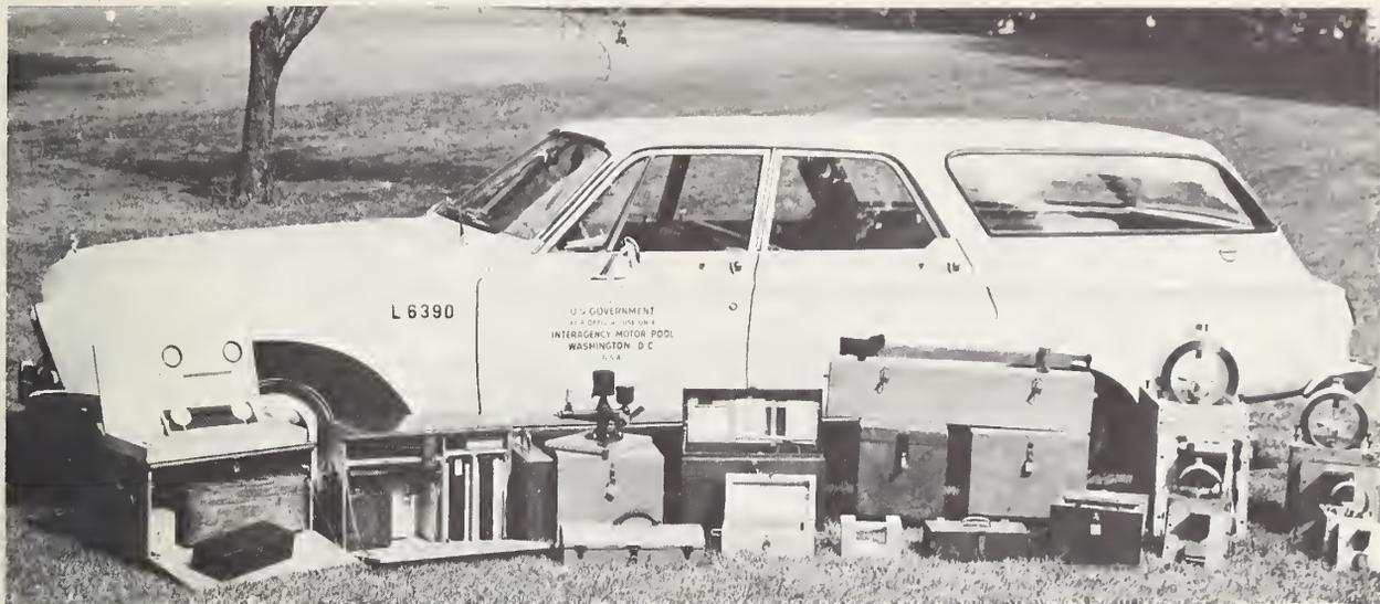
*The equipment employed by the NBS Cement and Concrete Reference Laboratory, sponsored by ASTM, to check test methods and apparatus used in cement and concrete testing laboratories throughout the United States and Canada.*
