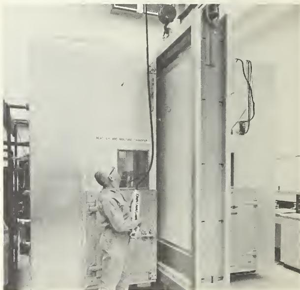
*An apparatus for studying air, moisture, and heat transfer through full-scale exterior wall constructions was composed of two environmentally-controlled chambers, open on their facing sides, capable of being closed with an airtight seal against a steel support frame for the wall specimen to be tested. A wall specimen is being moved into the apparatus by an overhead crane in this photograph.*
