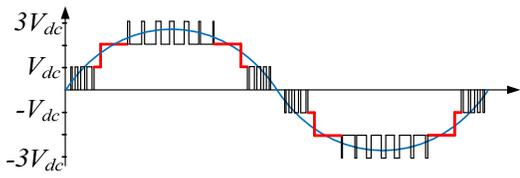
> Low freq. for high voltage module: loss reduction
