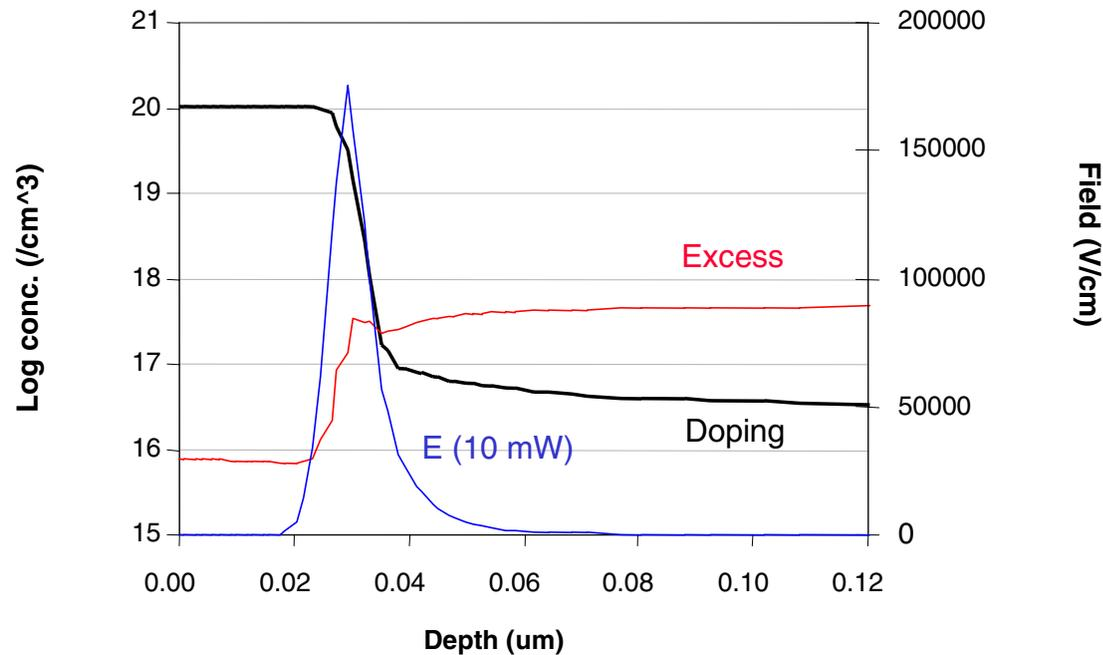
Steep rise in excess carrier concentration at junction edge.
