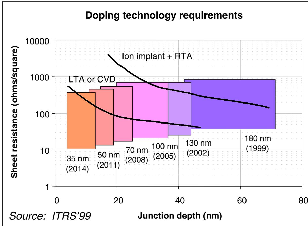
*USJ processes will be limited to a very narrow process window for depth, active dose, and uniformity*
