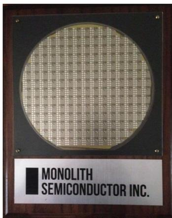
**First SiC power device fabricated in US on 150mm SiC wafers in a silicon CMOS fab**
