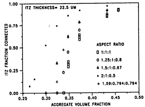
Figure 2: Percolated interfacial transition zone fraction vs. aggregate content. Three data sets are shown for the 1:1:1 aspect ratio system to provide some indication of variability.
