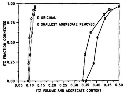
Figure 5: Percolated interfacial transition zone fraction vs. ITZ volume (dotted lines) and aggregate volume fraction (solid lines) for  $t=22.5 \mu\text{m}$  showing effect of removing finest aggregate particles.
