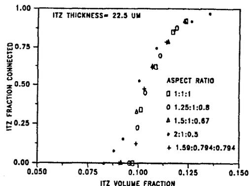
Figure 3: Percolated interfacial transition zone fraction vs. interfacial transition zone volume fraction.
