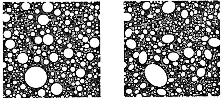
Figure 1: Two-dimensional slices from three-dimensional microstructures for aspect ratios of 1:1:1 (left) and 1.25:1:0.8 (right) (white: aggregate, grey: bulk cement paste, black: ITZ cement paste).
