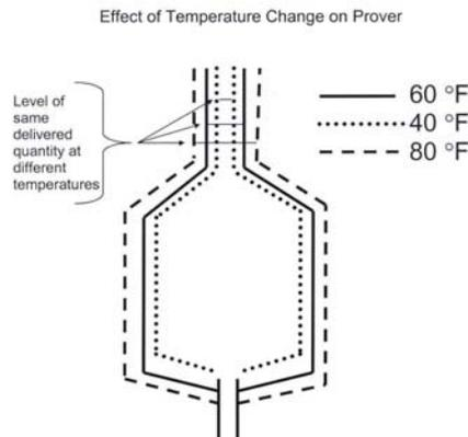
The common metals used for construction of volumetric field standards are mild steel and stainless steel. The accepted cubical coefficient of thermal expansion for the metals used to construct volumetric field standards is 0.0000186/°F for mild steel and 0.0000265/°F for stainless steel.
