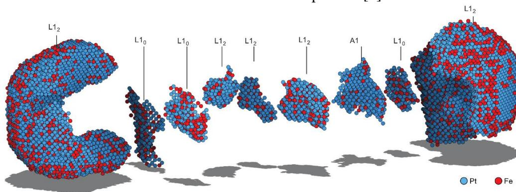
Figure 1. The nanoparticle consists of multiple FePt grains (type L<sub>1</sub><sub>0</sub> and L<sub>1</sub><sub>2</sub>) and a Pt-rich A1 grain.
