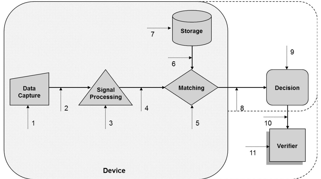
*This architecture stores biometric templates on an authentication device and requires that live samples be matched on that device. Once a match or no match result has been determined, the device sends the appropriate signal to the mechanism it is securing.*
