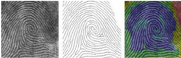
Figure 39 Examples of fingerprint, skeletonized representation, and overlay of original / skeleton / quality map
