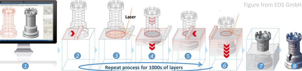
7. Remove 8. Post process to 6. Repeat 1. Create 3D 2. Apply layer 3. Solidify powder 5. Spread 4. Lower process for non-sintered create final part substrate by new powder of metal by melting with geometry powder on controlled laser 1000s of layer model usina one layer powder (heat treatment, machining, etc.) thickness CAD software substrate spot layers
