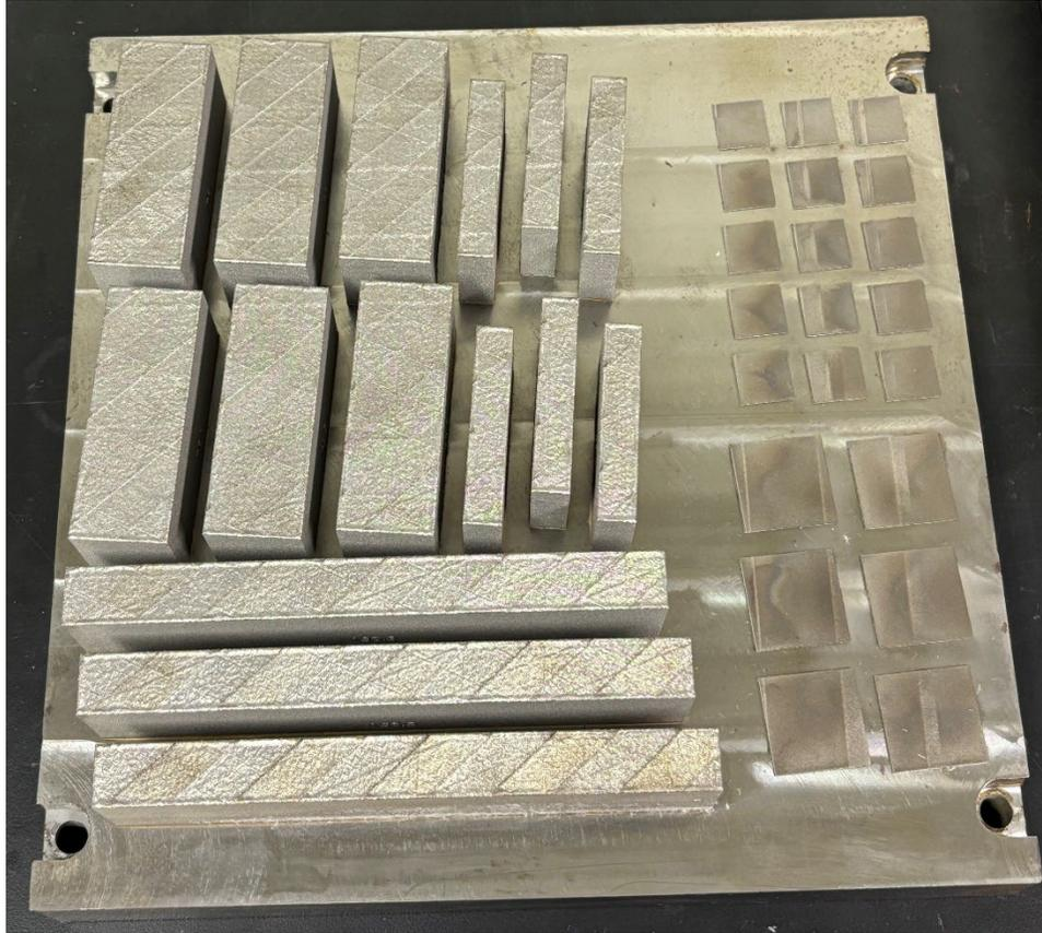
Figure 2. A photograph of a completed build plate with the '15.Y' and '25.Y' parts removed by EDM.
