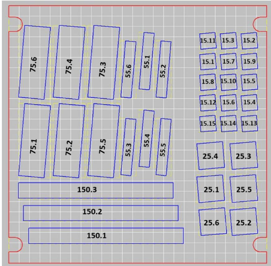
Figure 1. A schematic diagram of the build layout with sample labels overlaid with the sample geometries. The red outline corresponds to the build plate, while the blue outlines correspond to the part boundaries.
