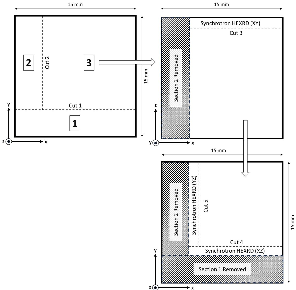
Figure 4. A schematic diagram for the sectioning of 15.Y parts to reveal different orientation planes for microstructural characterization. Note the sketch is not drawn to scale.
