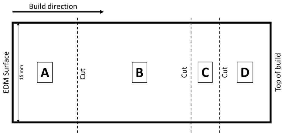
Figure 3. A schematic diagram for the initial sectioning of 15.Y parts along the build height. Note the sketch is not drawn to scale.
