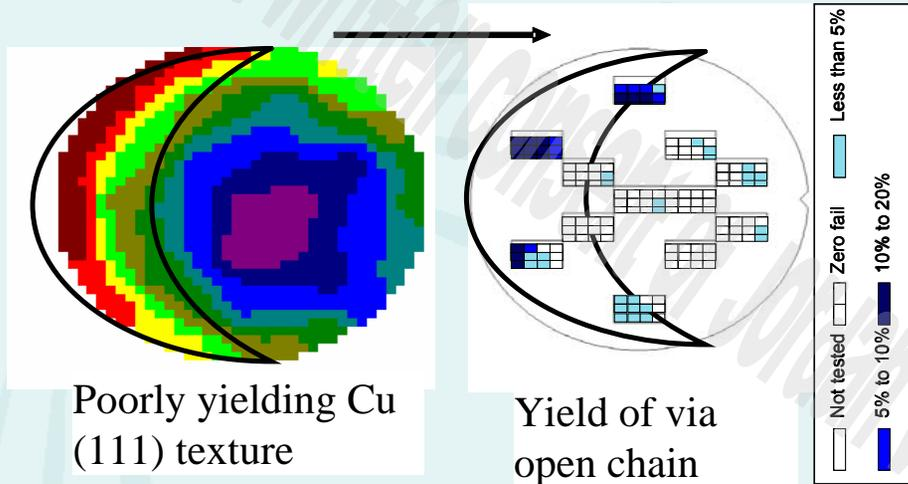
Cu Texture, i.e., non-random or preferred orientation of crystallites analysis of post-polish Cu establishes correlation of yield loss.
