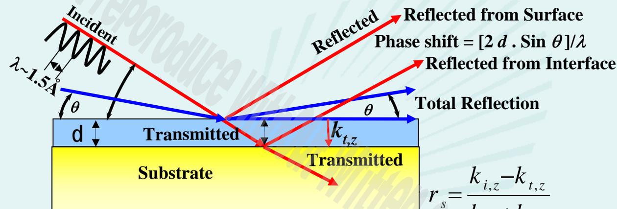
Reflectivity ( $r_s$ ) from any interface is calculated using Fresnel's equations employing continuity conditions for incident, reflected and transmitted waves.
