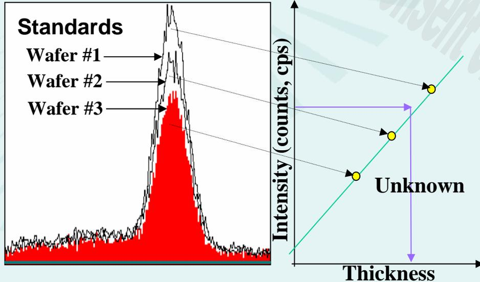
XRF Intensity is calibrated using known standards -
