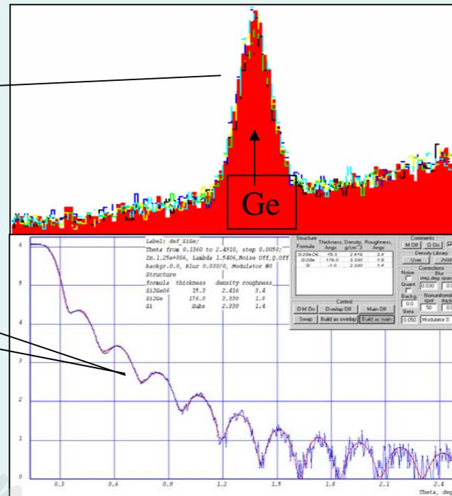
X-values for Si<sub>1-x</sub>Ge<sub>x</sub> using combined XRR and XRF data
