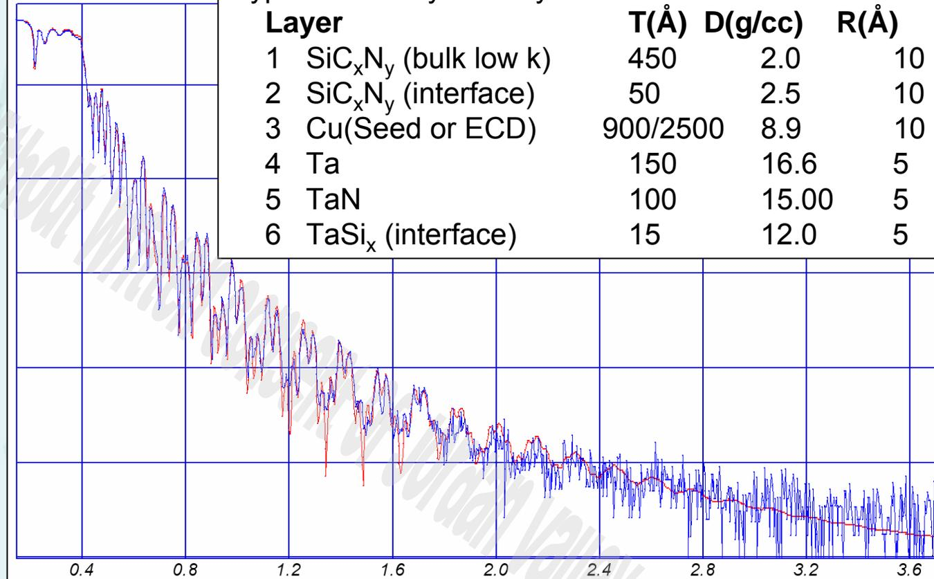
A single measurement can characterize a multi-layer stack
