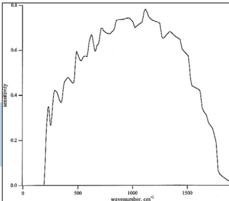
**Figure 31** The thermal infrared radiance emitted by the Earth's climate system has strong spectral features that resulting in substantial variation in radiant intensity within narrow spectral regions. The convolution of such rapidly varying features with unknown spectral response function structure is a potentially critical source of measurement error.
