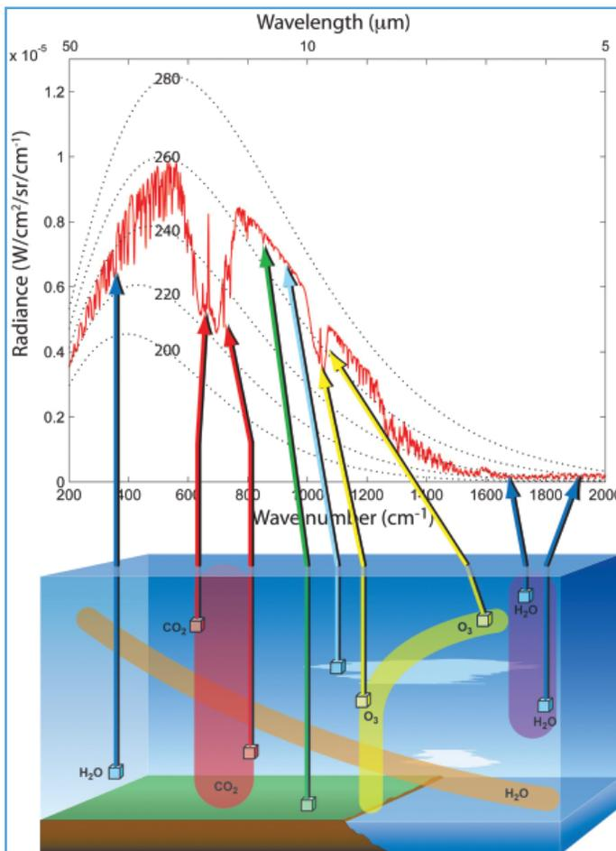
**Figure 3** The thermal IR spectrum. Frequency is in wavenumbers ( $\text{cm}^{-1}$ ), radiance in  $\text{W cm}^{-2} \text{sr}^{-1} (\text{cm}^{-1})^{-1}$ . Water vapor exhibits strong, narrow lines in the frequencies intervals 200–550 and 1100–1500  $\text{cm}^{-1}$ . Carbon dioxide absorbs in its  $\nu_2$  band in the frequency interval 550–770  $\text{cm}^{-1}$ . The area under this curve measures the flux of thermal IR energy radiated to space, thus cooling the Earth system.
