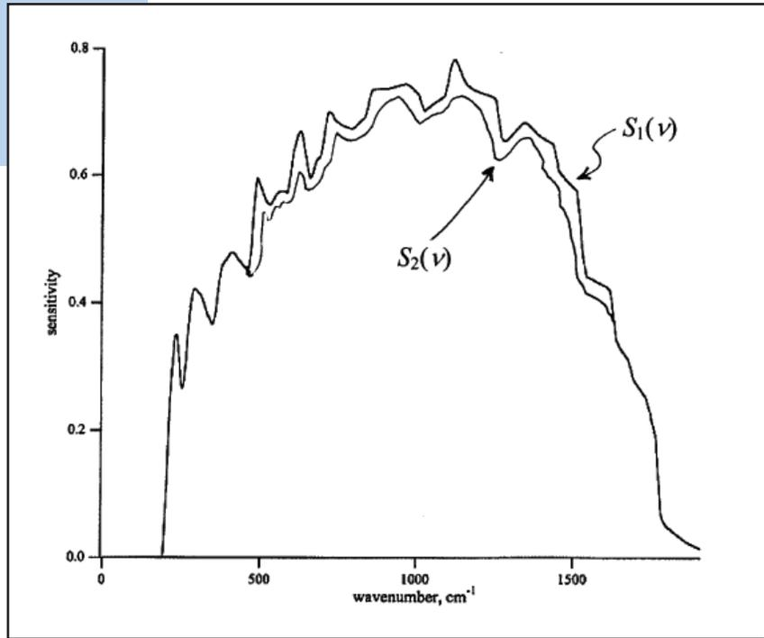
Because  $S(\nu)$  as a function of frequency cannot be uniquely determined on orbit with a broadband instrument, it is impossible to establish the (small) changes in the key quantity  $I(\nu)$  as a function of time. In sharp contrast, the spectrally resolving instrument, by design, has the intrinsic capacity to establish the spectral response function,  $S(\nu)$ , on orbit. It does this in the following way:
