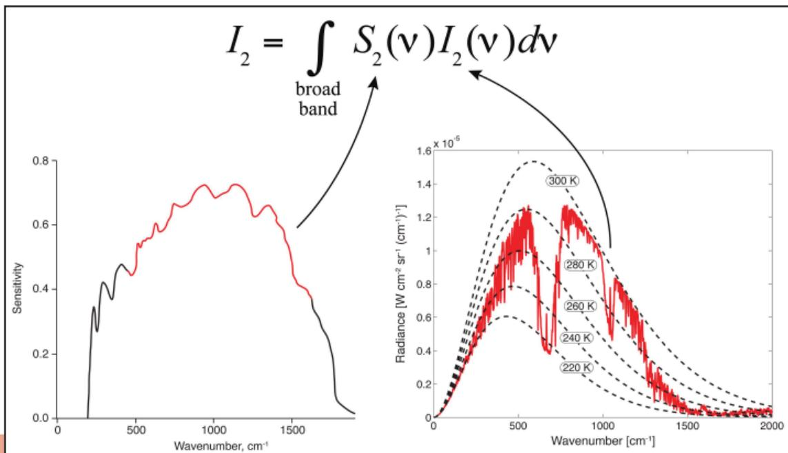
**Figure 33** Aging due to environmental exposure causes alteration of the radiometer spectral response function. Since the unknown climate change signal is convolved with this unquantified change in spectral response function, definitive detection and interpretation of climate change is out of reach.
