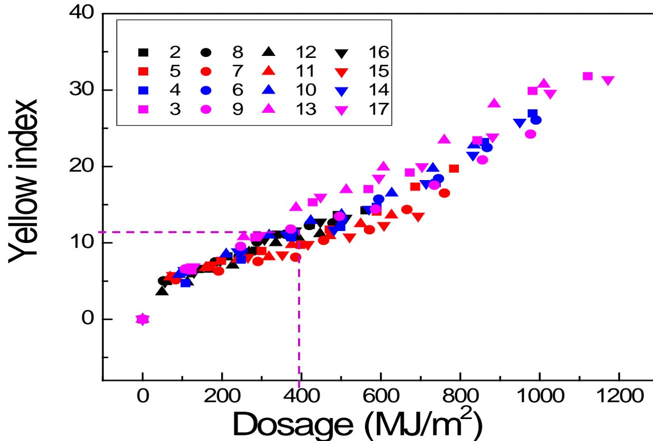
For a given damage, the required dosage is similar at different light intensities.
