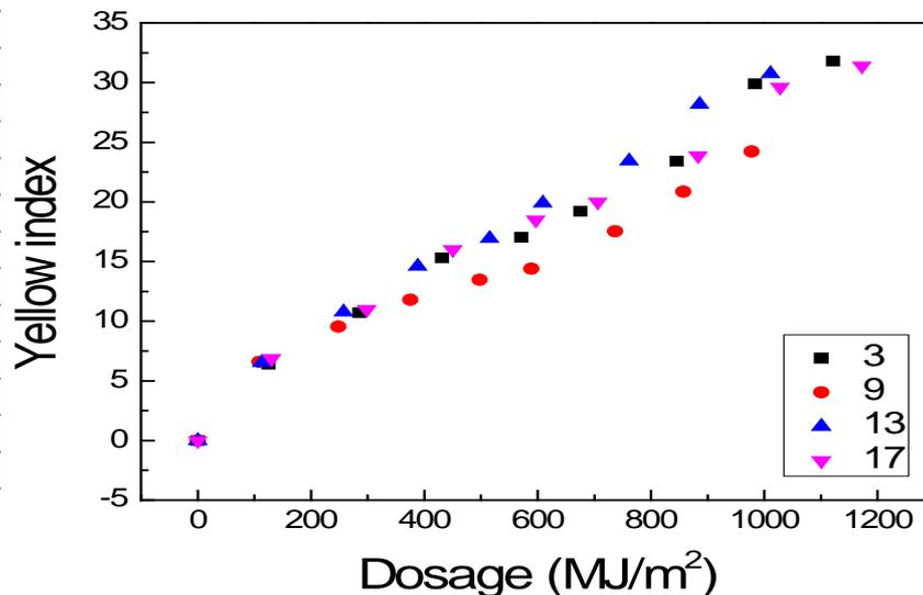
The data from the replicates are generally consistent; the deviation could be due to the non-uniformity of the EVA curing and the EVA thickness.
