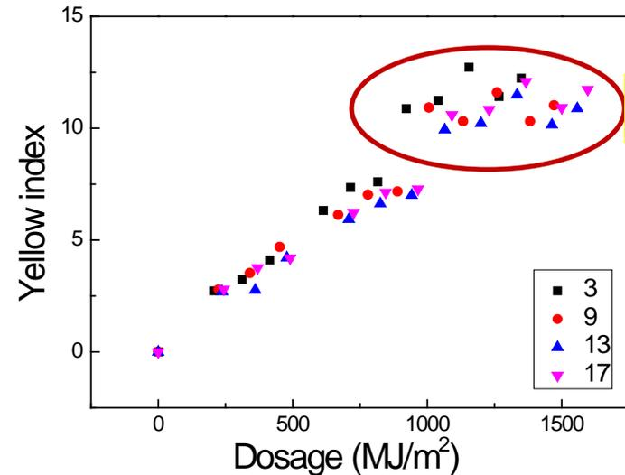
The data from the replicates are generally consistent; the deviation could be due to the non-uniformity of the EVA during curing.
