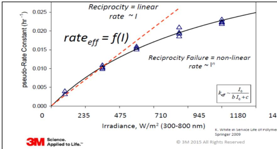
Pseudo-rate constant is defined as the **slope of yellow index vs. time** curve in this study (Assuming a linear relationship between yellow index and aging time)
