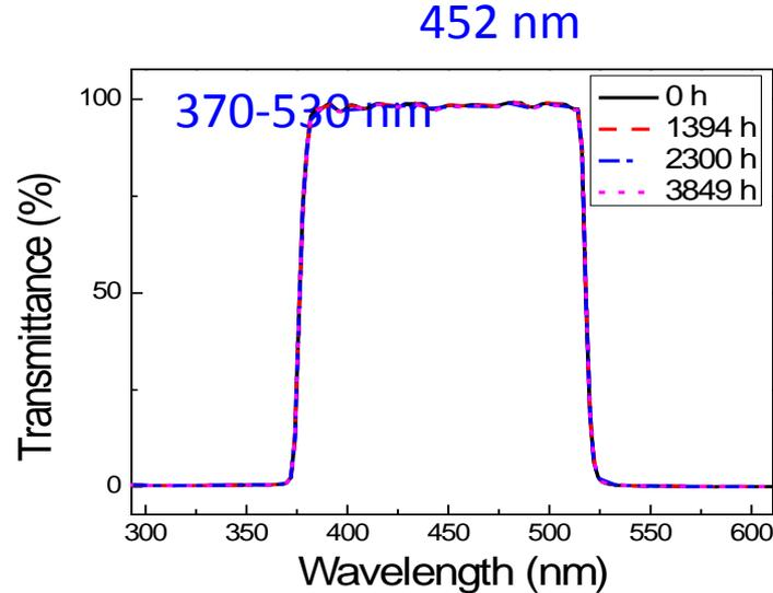
No obvious changes have been observed for these band pass filters at 85 °C/0 % RH on the SPHERE so far.
