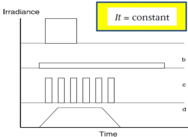
Figure 1—A selection of radiant flux versus exposure time regimes for testing the law of reciprocity in which the dose (integrated area on plot) for each exposure regime is identical. Assuming that the reciprocity law is obeyed, then the photoresponse for each of these exposure regimes should be the same (adapted from reference 6).
