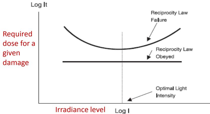
Figure 2—Kron's graphical method for presenting reciprocity data in which the logarithm of dose (irradiance x time) necessary to produce a given photoresponse is plotted against the logarithm of irradiance (adapted from reference 13).
