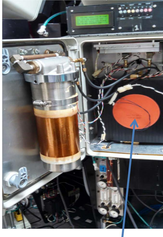
Sample cover with heating pad. The sample is held inside.
