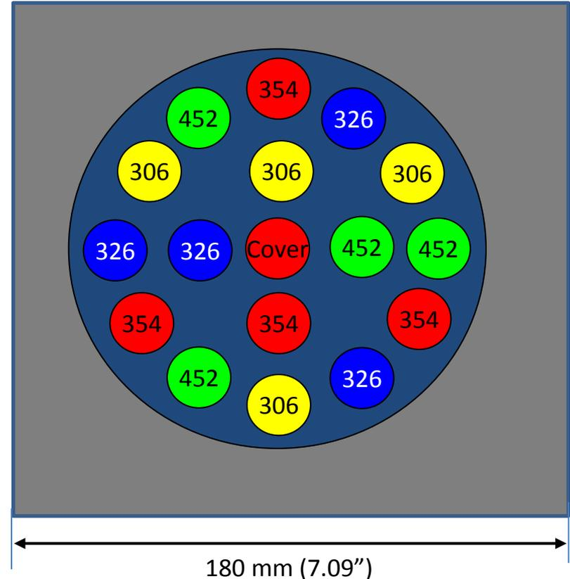
Varying **wavelength** range with narrow band pass filters,  $(306 \pm 3) \text{ nm}$ ,  $(326 \pm 6) \text{ nm}$ ,  $(354 \pm 12) \text{ nm}$  and  $(452 \pm 24) \text{ nm}$ .
