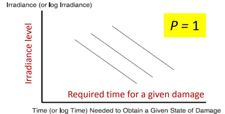
Figure 3—Plot of irradiance (or log irradiance) versus time (or log time) needed to achieve a given photoresponse (adapted from reference 17).
