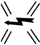
Heat Switch: the switch disconnects power to the heating elements; unless this switch is off there is a danger of electric shock when inserting objects into the furnace
