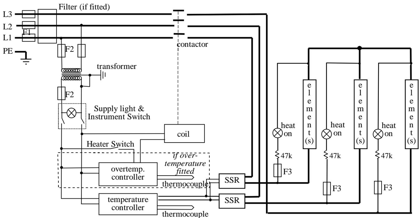
Note: in this configuration the fuses F2 on the supply side of the transformer may be GEC Safeclip, not 32 x 6mm glass as stated in section 8.1.
