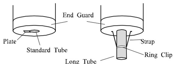
**Fig.1. - Vertical Tube Retention**
