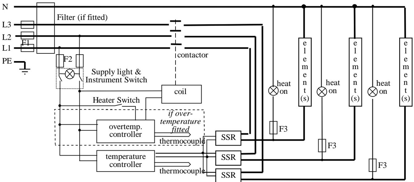
note on (2- and) 3-phase: depending on filter(s) fitted, there may be (2 or) 3 separate neutral wires from the elements to the neutral supply.
