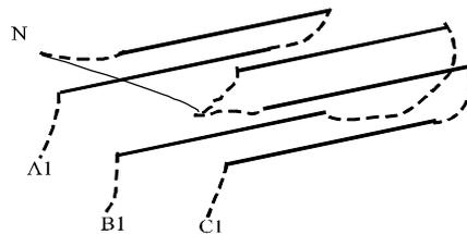
Fig.8. - Element Connections - 6 elements, 3 phase
