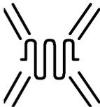
Heat Light: the adjacent light glows or flashes to indicate that power is being supplied to the elements
