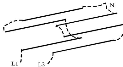
Fig.7. - Element Connections - 6 elements, 2 circuits
