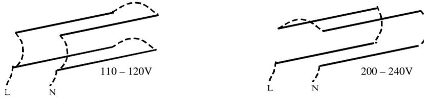
Fig.6 Element Connections - 4 elements
