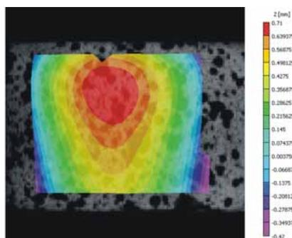
DIC Measurement of Tissue Simulant Material
