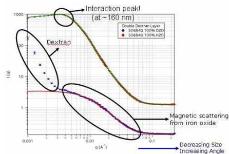
Small angle neutron scattering data showing interactions.
