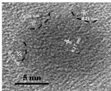
TEM image of Co nanoparticle, with dotted lines showing location of CoO patches.
