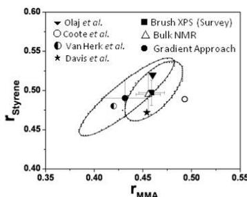
Reactivity Ratios for Styrene Methyl Methacrylate Polymerizations measured from a copolymer library fabricated in a microchannel
