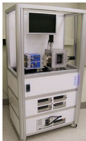
The high temperature TE metrology apparatus under construction.
