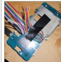
This is an Android HTC mobile phone that is wired up for the JTAG process.
