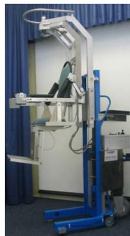
**Figure 3 – HLPR Chair prototype shown in the patient lift position.**
