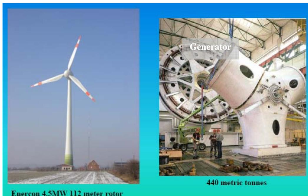
Fig. 6. Photograph of the Enercon 4.5MW wind turbine. The generator and hub weight 440 tonnes, compared to an estimated 118 tonnes for an 8MW HTS design.[6]
