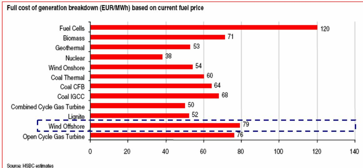
Fig. 5. Comparison of Cost-of-energy (COE) among various power generation technologies. Presently, offshore wind costs 46% more than onshore wind. [5]
