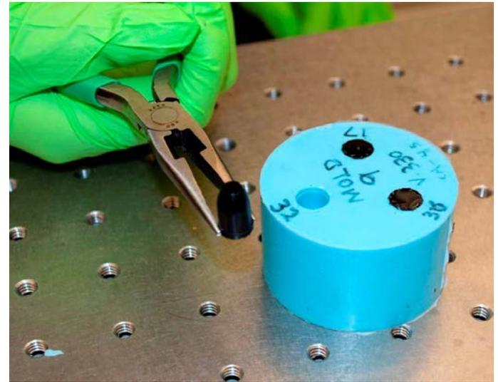
Carefully separate the silicone from the urethane replicas and then remove the replicas with needle nose pliers. The bullet standoff in the replication rig will avoid contact with the striated regions of the bullets, avoiding any damage.
