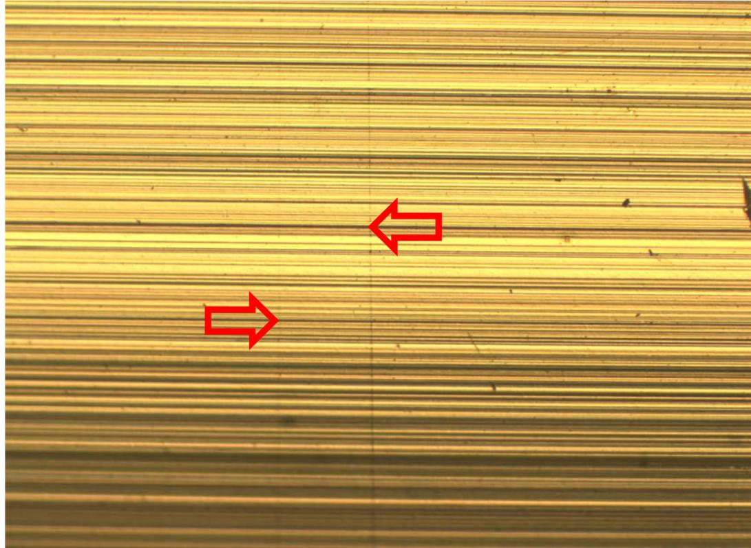
**Even stylus traces from original SRM 2460-038 are visible in the replication. These features are sub-micrometer in scale.**
