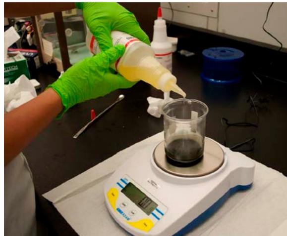
Mixing polyurethane with dye, and vacuum-degas
