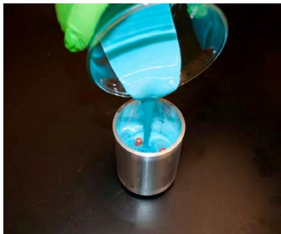
Pouring silicone into replication rig
