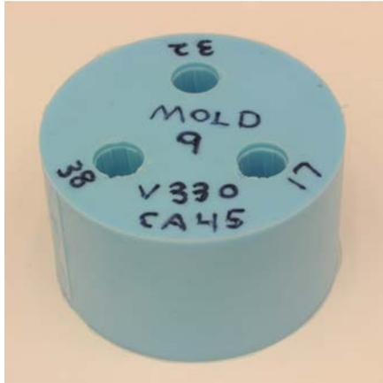
Multiple replicas made from a single mold.
