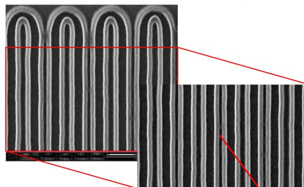
Over 200 fast-scan 512 pixel by 480 pixel, 100 ns dwell time images are added together (averaged) using 2D Fourier transform to compensate for drifts. The resulting raw images were used as input for the model-based 3D evaluation of the lines. Quadruple exposure "fin-FET" structures of approximately 10 nm wide lines (Intel).
