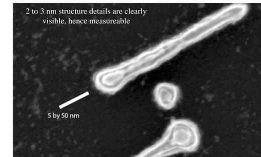
Even top-down images reveal a tremendous amount of 3D information. Here 3D structure is clearly visible, so is the residue on the surface. Top-down view of a resist sample of intentional defect arrays
