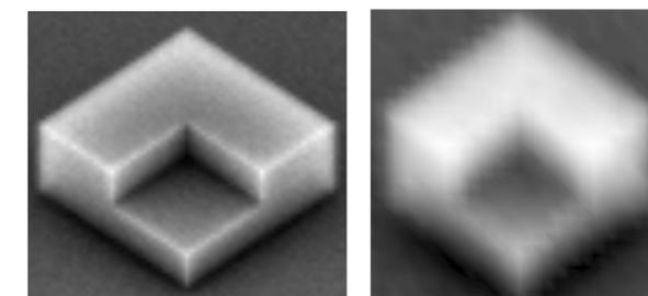
3D simulation of complex structures for the assessment of likely SEM images. Note the meaningful 2D and 3D edge effects, the lower secondary electron yield at the inner corner and at the edges sitting on the substrate. 1 keV landing energy, 40 nm wide, 20 nm tall, 0.5 nm beam spot size (left) and 6 nm wide, 3 nm tall, 0.3 nm beam (right) structures
