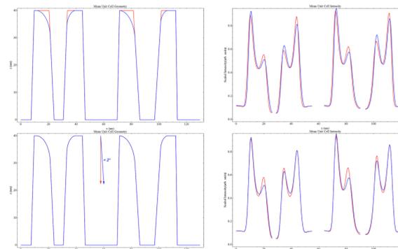
The relationship among of the shape and their corresponding waveforms (top); the difference between the waveforms with and without tilted primary electron beam (bottom)
