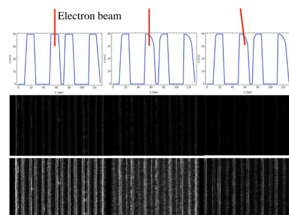
The various shape approximations and their results. The left, middle and right shows these for trapezoidal, "shark fin" and "shark fin" with "stray tilt" respectively at the top, and their corresponding actual differences (at the center) and the differences amplified to show the residues clearer (at the bottom)
