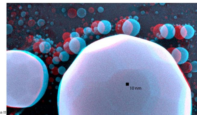
3D SEM measurements of complex structures is possible by acquiring two or more images from different viewpoints, and by using a suitable rendering software
