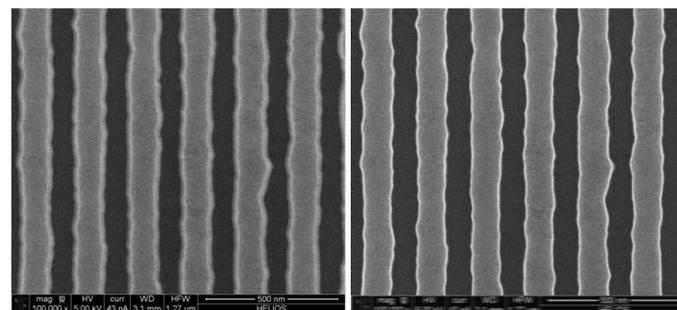
The traditional fast imaging results in blurry images (left) The NIST 2D Fourier-transform-based image acquisition method compensates for drift and provides more accurate image (right).
