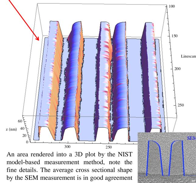
An area rendered into a 3D plot by the NIST model-based measurement method, note the fine details. The average cross sectional shape by the SEM measurement is in good agreement with TEM image (Intel).
