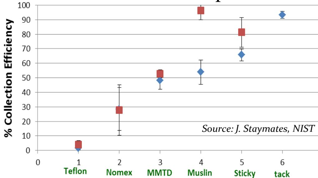
Wipe material, surface characteristics, particle size, applied force - all significant factors
