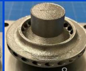
AMPed LOX Impeller Iterations
