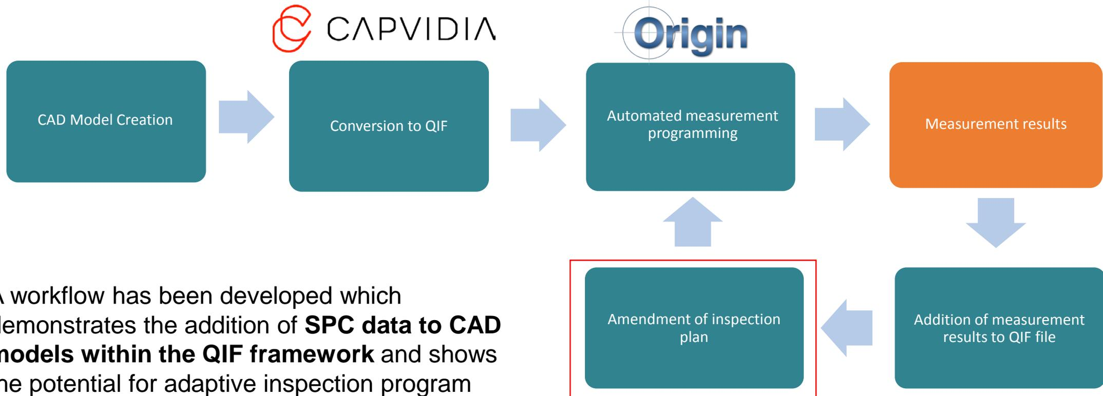
A workflow has been developed which demonstrates the addition of **SPC data to CAD models within the QIF framework** and shows the potential for adaptive inspection program changing based on these results.
