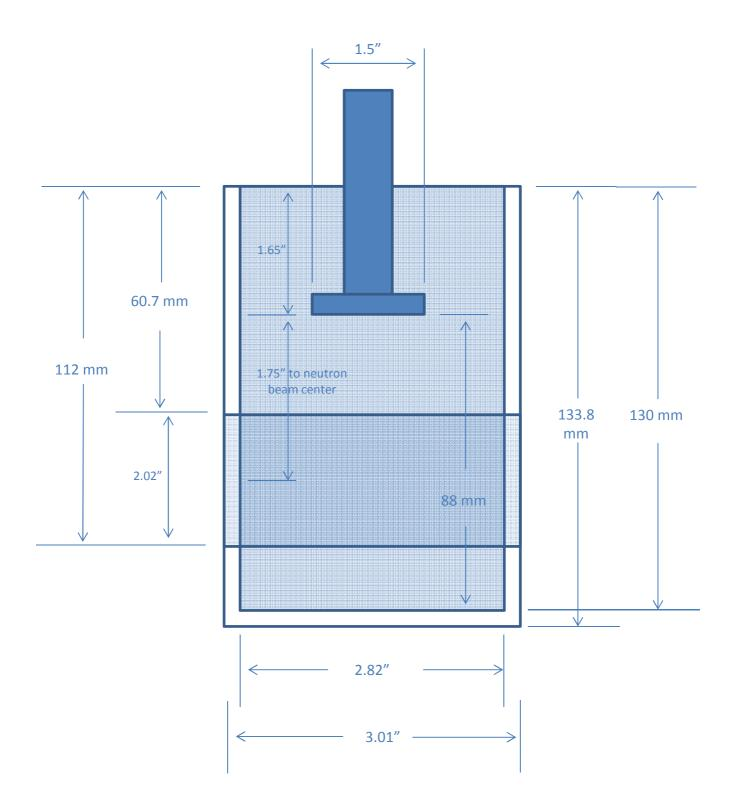
There is 2 mm space between the top of IVC and top of the taper part. The center of sample needs to be 1.75" below the mounting flange. Maximum length is 86 mm. Otherwise touching the IVC bottom. Active length is 19-70mm. Sample diameter < 70 mm (the smaller the better) with a 5/16-18 bolt less than 1/4" long on top of it. We also may need to make centering jig out of nylon because the mounting flange wiggles a little and is NOT centered to great precision.
