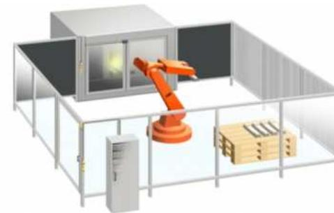
Traditional robot workcell setup
