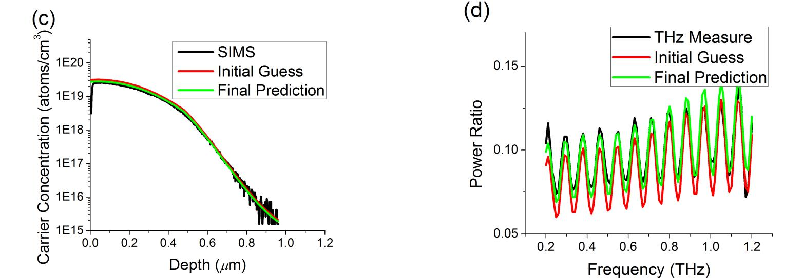
Demonstration of doping profile prediction with initial guess profiles from TCAD and its comparison with the SIMS measurements for (a,b) ion implanted, rapid thermally annealed with a dose of 1x10<sup>15</sup> cm<sup>-2</sup>; (c,d) thermally diffused with a dose of 2x10<sup>15</sup> cm<sup>-2</sup>.
