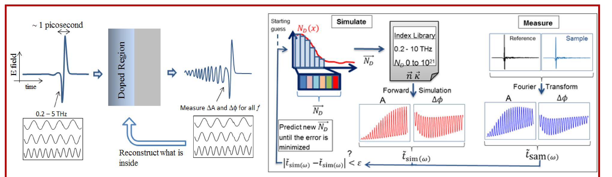
Schematic of the algorithm that solves the inverse problem of mapping unknown doping profiles. The algorithm inputs are measured amplitude and phase data and it also needs a real and imaginary index library.
