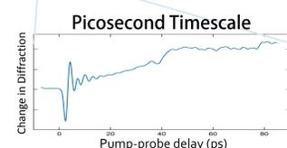
We focus an ultrafast laser onto a nano-patterned ultrathin film and substrate, causing thermal expansion and launching both surface acoustic waves (SAWs) and longitudinal acoustic waves (LAWs). EUV pulses probe the propagation dynamics of both SAWs and LAWs enabling the characterization of both Young's modulus and Poisson's ratio in a single measurements, as well as nanoscale heat dissipation rates.
