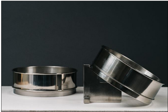
Figure 2-3. Sieve with Tilt Block Set at 30 Degrees
