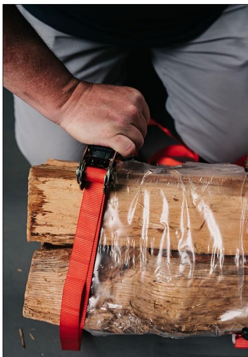
Figure 3-16a. Strapping the Ends of a Bundle
