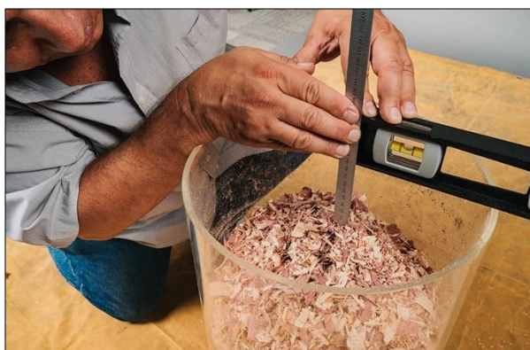
Figure 3-31. Reading the Depth of the Container
