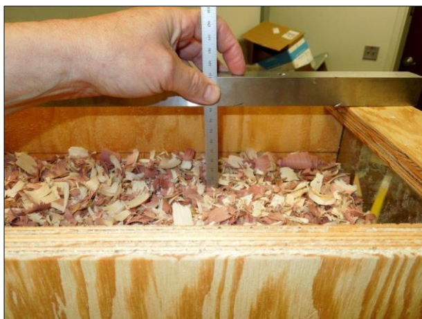
Figure 3-37. Using the Headspace Measurement on 56.6 L (2 ft³) Test Measure
