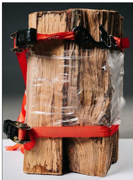
Figure 3-17. A Tightly Wrapped Bundle with Straps Placed at 10 cm (4 in)
