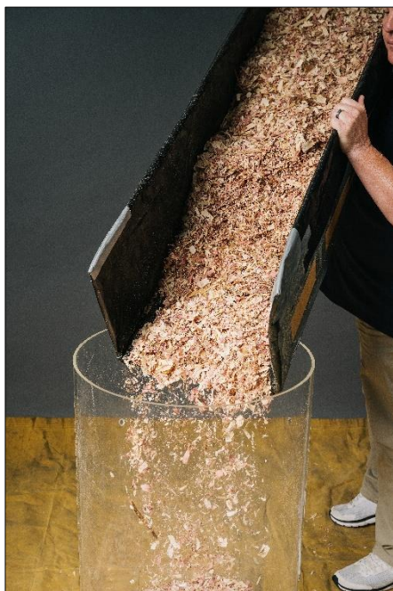
Figure 3-26. Filling a 44 L Test Measure
