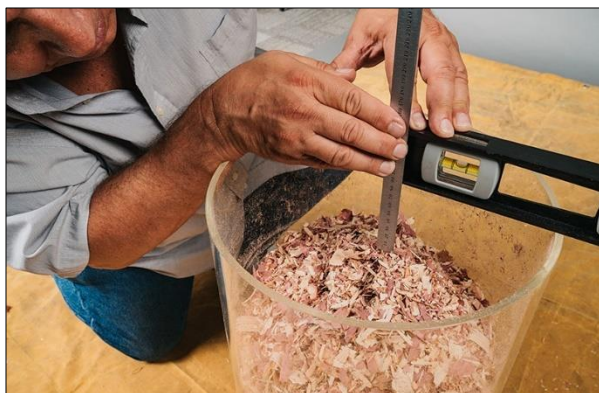
Figure 3-31. Reading the Depth of the Container
