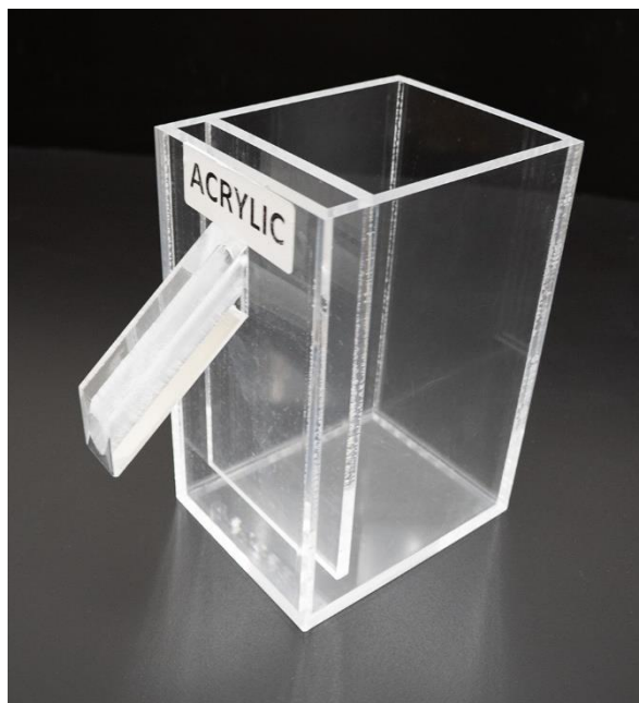
Figure 3-7(a). Example of a Displacement Vessel
