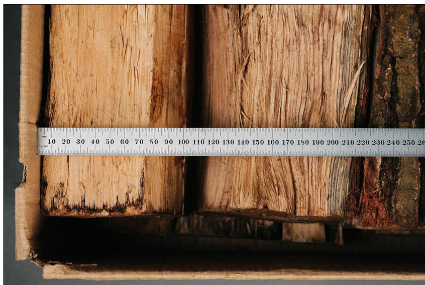
Figure 3-10a. Measuring the Width of the Firewood in a Box
