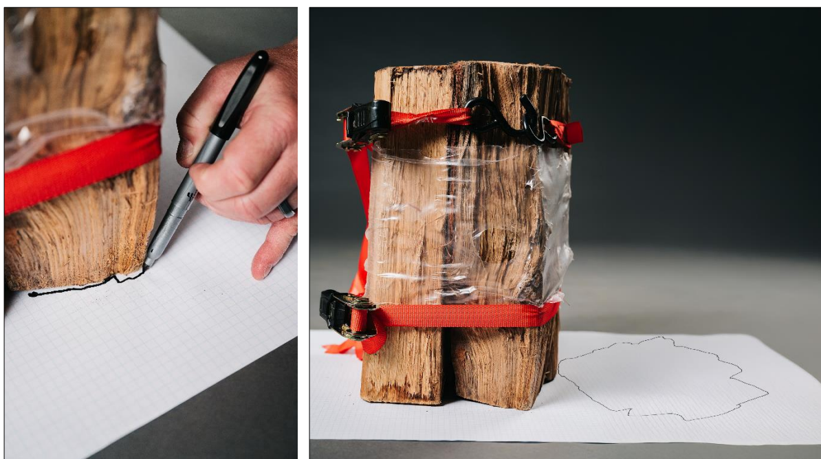
Figure 3-18a and 3-18b. Tracing the Perimeter of the Wood
