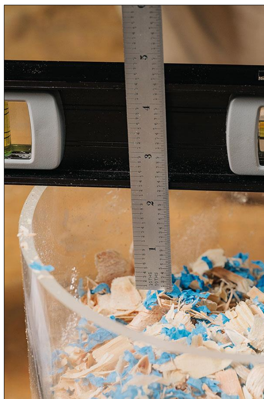
Figure 3-30. Ruler Shown with the Zero End at the Bedding Surface
