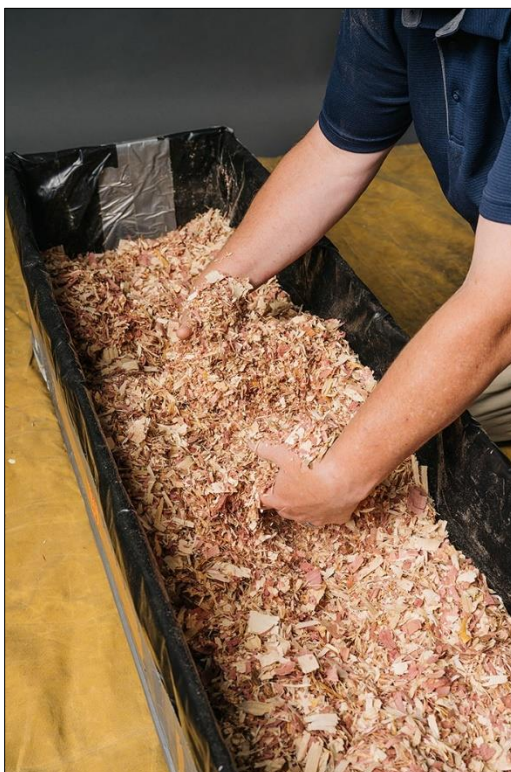
Figure 3-23. First Pour into the Test Measure
