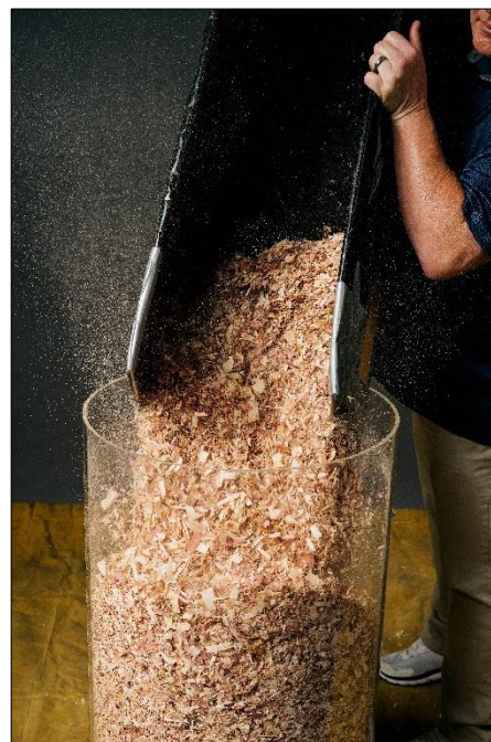
Figure 3-27. Filling a Test Measure at an Angle to Use the Larger Opening
