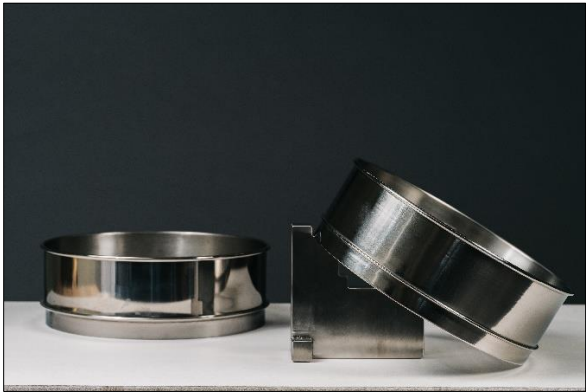
Figure 2-3. Sieve with Tilt Block Set at 30 Degrees
