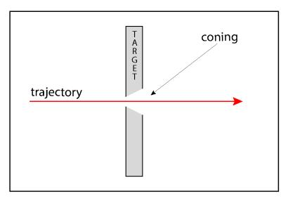
**Figure 5:** A cross-section of a projectile perforation through a brittle material that shows the orientation of the *cone* (3.27) with the larger diameter side on the exit surface.
