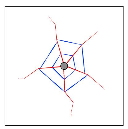
**Figure 7:** Concentric fractures (3.26) (shown in blue) are oriented in a generally circular form around the impact site. Radial fractures (3.65) (shown in red) that extend outward from the impact site.
