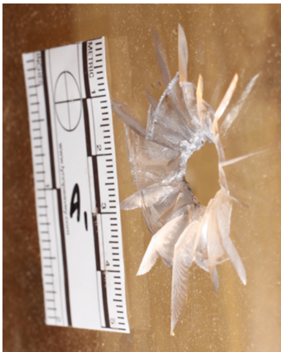
Figure 6: A projectile perforation through a brittle material (plexiglass) that shows the orientation of the cone (3.27) with the larger diameter side on the exit surface.
