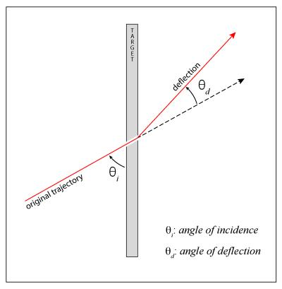
**Figure 1:** A projectile perforation that shows the original trajectory which forms the *angle of incidence* (3.4) with the target surface and the deflected path of the projectile that forms the *angle of deflection* (3.3) with the unaltered path (dashed line).
