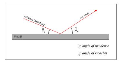
**Figure 2:** A projectile ricochet that shows the original trajectory which forms the *angle of incidence* (3.4) with the target surface and the deflected path of the *ricochet* (3.xx) that forms the *angle of ricochet* (3.5) with the target surface.
