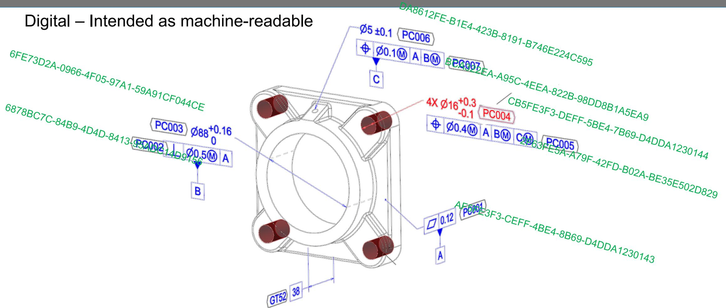
Representation of a Model-Based Definition with Product Characteristic Reference Tags & UUIDs
