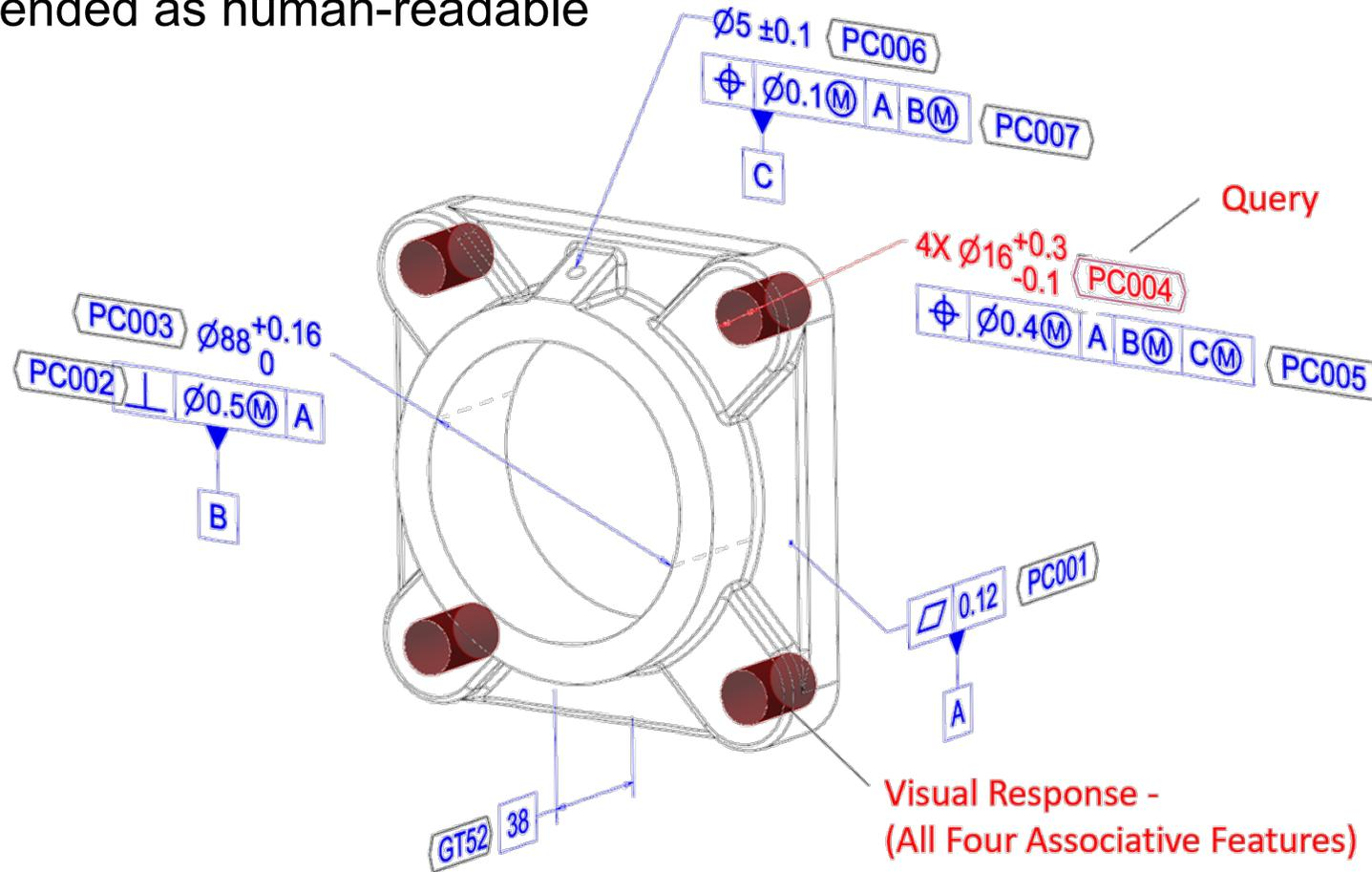
Visualization of a Model-Based Definition with Product Characteristic Reference Tags
