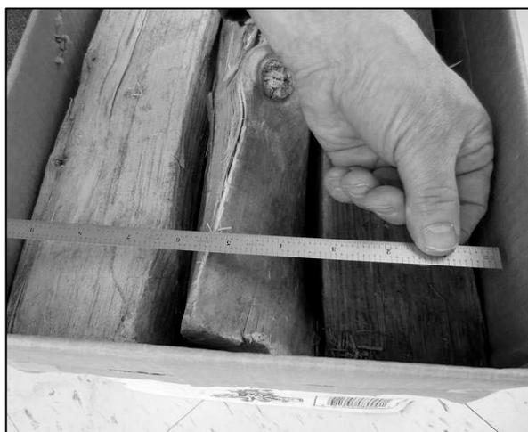
6. Individual Piece Length. Remove the wood from the package and measure the length of each piece of wood (see Table 3-5. “Minimum Number of Pieces to be Measured for Length”). If the piece of wood is uniform in shape, take at least one point-to-point measurement along the center line of the longitudinal axis (see Table 3-6. “Determining Piece Length, (a) Uniform Shapes” for examples) and record the value.
