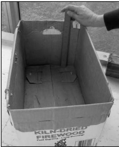
**Figure 3-8. Measuring the Internal Height of the Box.**
